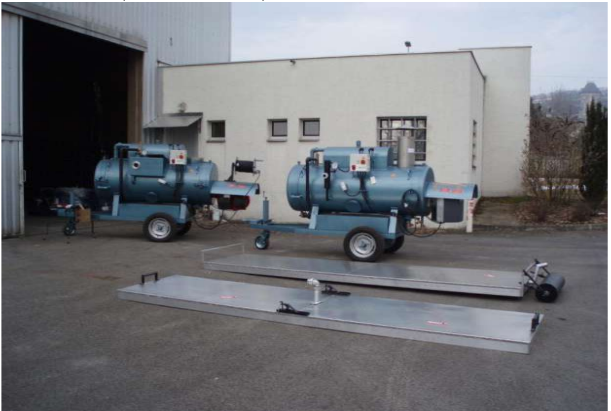
Agrivap 2006 and one Agrivap 2004 and 2 cloche covers one prepared for POL system and one with rear roller (the roller is retractable)
